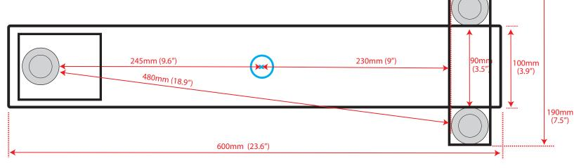
For use with hydraulic cylinder 125kN capacity or Model 2008 Tester
