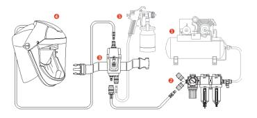
Air is compressed outside of the hazard area (1) and is channelled to a coalescing Filter (2) to be cleaned. From the filter (2), the air passes to the respirator waistbelt (3), where it is regulated to a constant flow. Air then reaches the visor (4) to provide the operator with breathable quality air. It also supplies air to the air tool (5).
