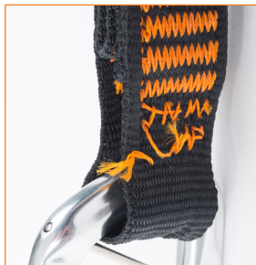
Activated shock absorber: please notice the torn stitching. For a correct control you must check the condition of the webbing and of the stitching below the protection sheath.
