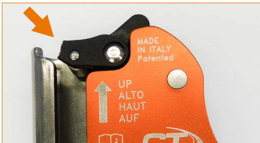
Broken safety lever.
