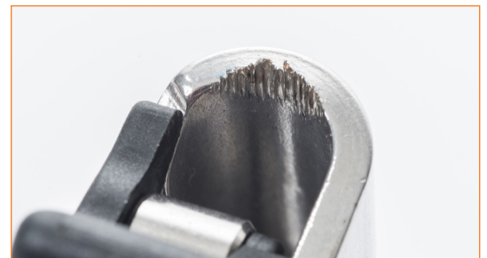
Device that has arrested a fall: edge of the body having incisions caused by the sliding of the cable.
