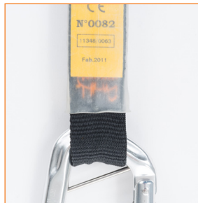
Activated shock absorber: please notice the torn stitching. For a correct control you must check the condition of the webbing and of the stitching below the protection sheath.
