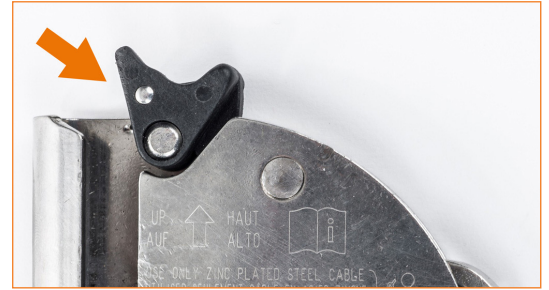
Safety lever that doesn't return autonomously into position.
