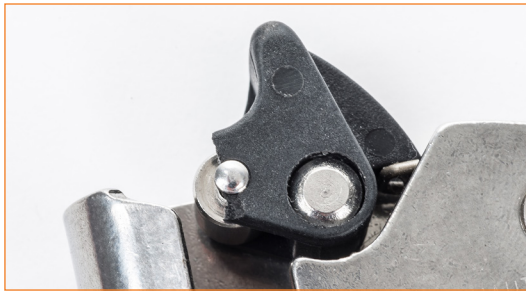
Damaged safety lever.
