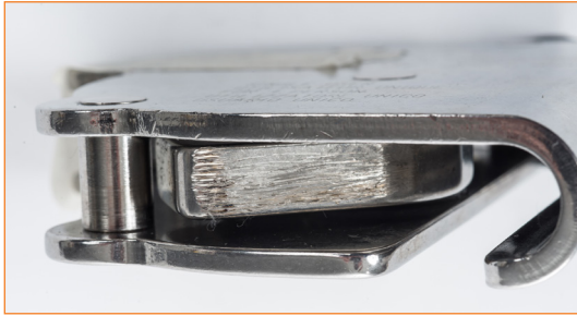
Device that has arrested a fall: blocking cam having incisions caused by the sliding on the cable.
