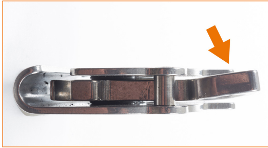
Bended locking cam.
