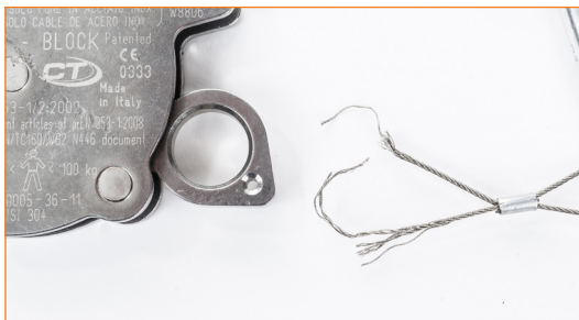
Broken connecting cable.
