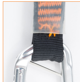
Activated shock absorber: please notice the torn stitching. For a correct control you must check the condition of the webbing and of the stitching below the protection sheath.
