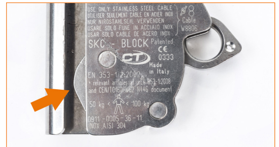
Locking cam that doesn't return autonomously into position.
