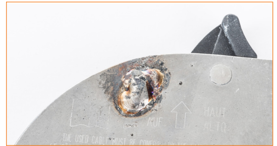
Welding sign close to the rivet.
