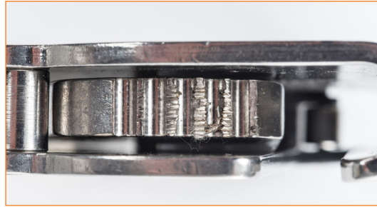
Device that has arrested a fall: blocking cam having incisions caused by the sliding on the cable.
