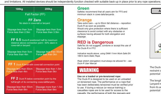
The Duck-R has successfully been tested by the manufacture to with loads of 200kg for rescue purposes. This testing is designed to replicate rescue techniques and requirements with limited lanyard lengths and limited Fall Factors. The testing produced provided consistent performance
