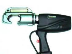
Die for 8mm cable for battery powered crimping tool.
