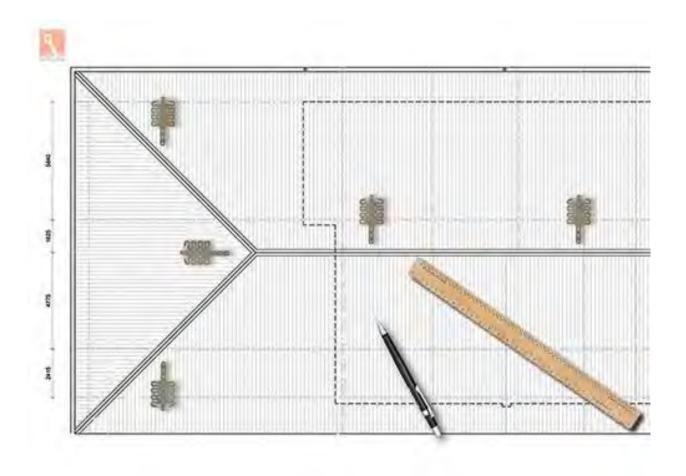
SafetyLink's design and planning team are here to help work out the positioning of your fall protection system, ensuring all areas of your roof are accessed safely.
