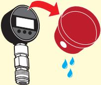
**If equipment has been used in very wet weather it is advised to peel back the outer rubber casing and leave to dry out before next use.**
