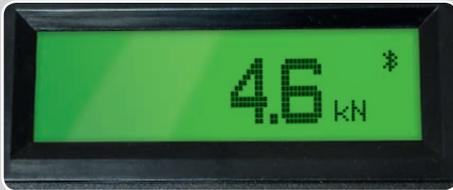
When connected the Bluetooth symbol will stop flashing and remain on.
