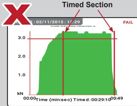
The timer was left to run during the wind down. The app result is performed on the results between the timed section (when wind down load was below target) and so produces a FAIL.
