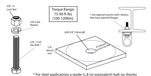
Swivel anchor must be flush with steel surface. A 16mm bolt may be used in place of a 5/8"-11 for metric applications.
