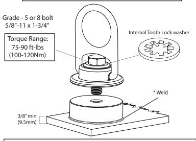
\* Welding procedure must be approved by an Engineer or other qualified person to be compatible with any and all structural & operational characteristics of the selected installation location.
