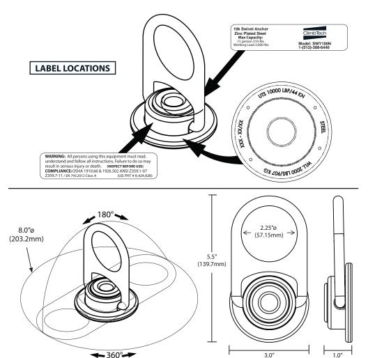
Tensile Strength (UTS): 10,000-lbf (44kN)
