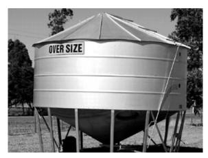
1. Field bin that incorporates sight glasses for showing product level and a fill hatch operated from the ground.
