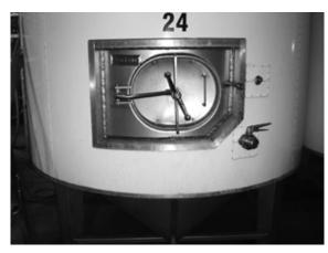
2. Vats with inlets, outlets and controls near ground level.
