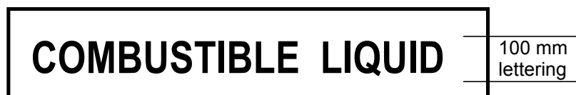
Figure 13.5 Placard for C1 combustible liquids
